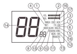
Figure 3-3 LCD Display Layout
